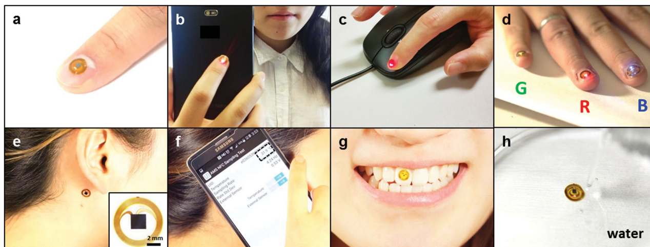
Figure 5. Pictures of various points of integration of mm-NFC devices on the body, each suggestive of a different application possibility. a) Picture of a device on the fingernail. Pictures of applications to unlock b) a smartphone and c) computer (using a mouse). d) Picture of a set of devices with integrated LEDs mounted on the fingernails. e,f) Pictures of a device mounted on the skin behind the ear, with integrated temperature sensing capabilities. Inset: Picture of a device that enables temperature sensing. Pictures of devices g) on a tooth and h) submerged in water.
