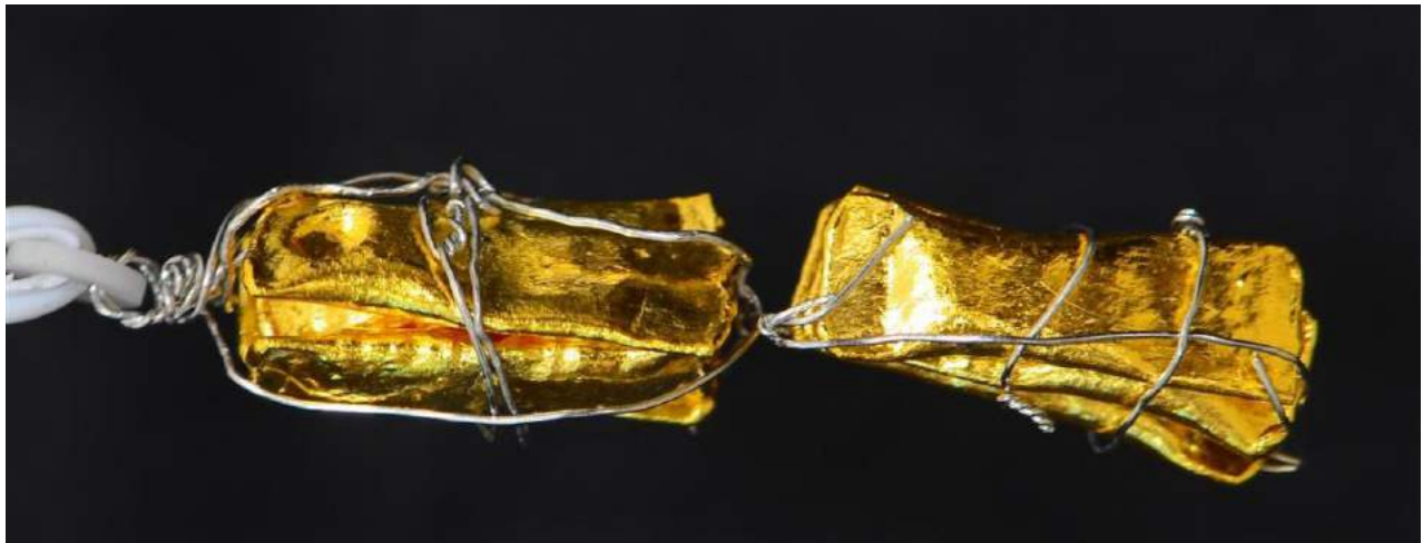
The samples subjected to temperatures of 1,000-1,040°C source - kuleuven.be
