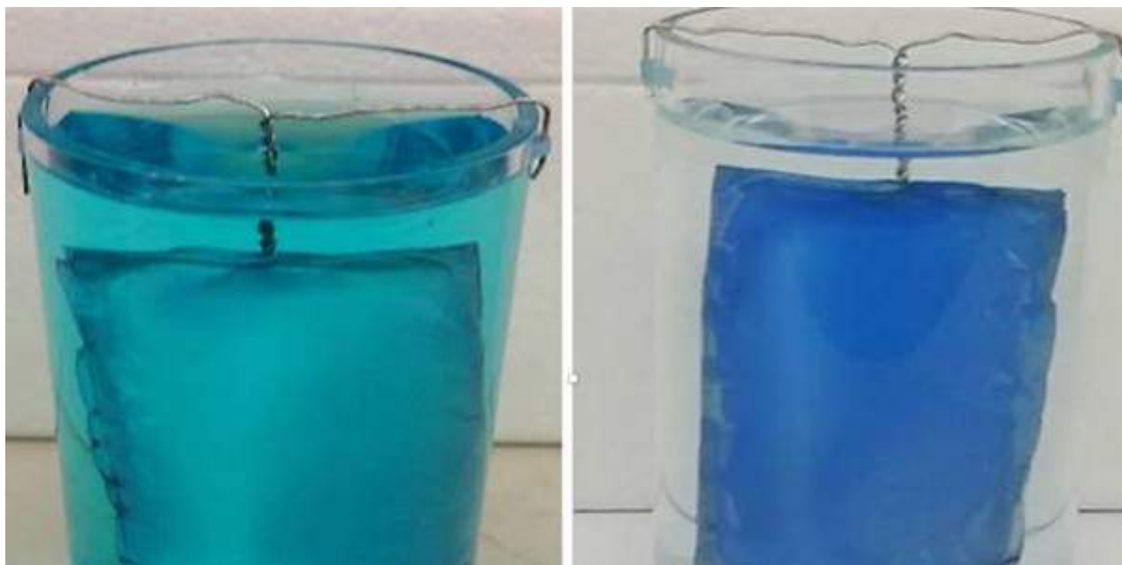
A mat is immersed in water with methylene blue as a contaminant source - rice.edu
