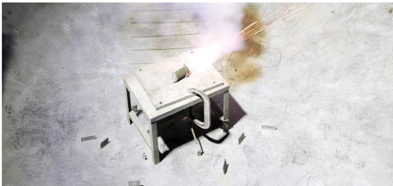
A new type of smoke grenade that can obscure sensors in the visible and infrared ranges burns during a test source - acs.org
