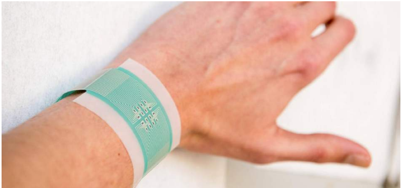
The sensor array is designed to draw fluid across a single hair follicle source - bath.ac.uk
