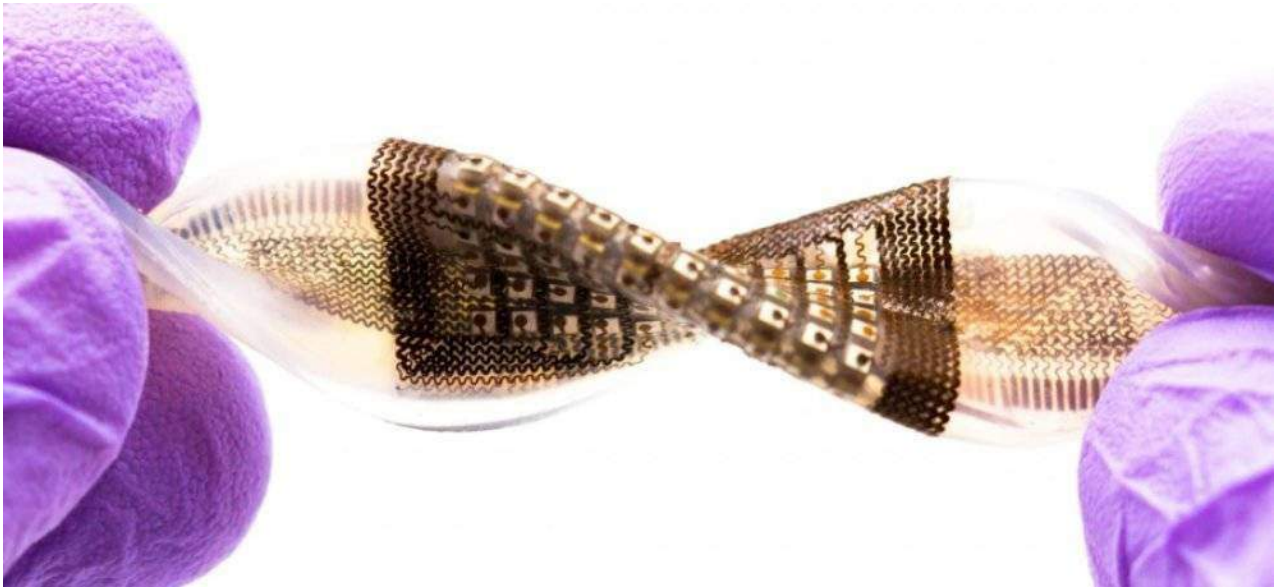
The patch could make it easier to inspect damage deep inside odd-shaped structures source - ucsd.edu
