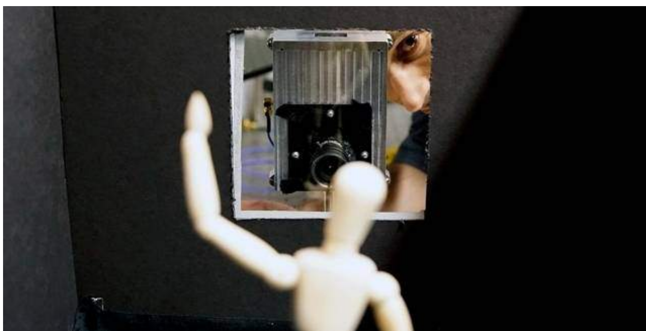
The system was able to resolve images of objects and gauge their depth at a range of 57 centimeters source - mit.edu
