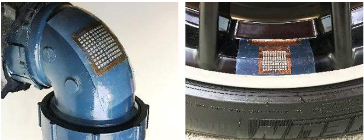
The patch can easily conform to odd-shaped surfaces such as pipe elbows and wheel edges source - ucsd.edu
