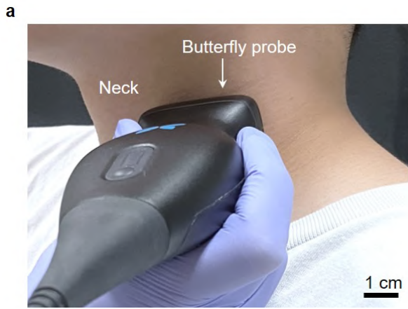
Supplementary Fig. 27 | The long-term skin integration comparison between a, a commercial Butterfly system (the benchmark of cellphone based portable ultrasonic systems) and b, a stretchable phased array demonstrated in this work.
