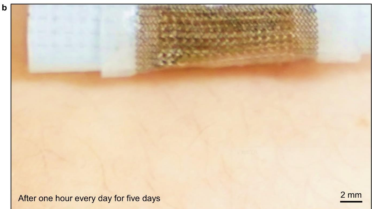
Supplementary Figure 51. Optical images of skin before and after monitoring. The device was mounted on the upper arm one hour every day for five days. No obvious skin irritation occurs, showing that the device is appropriate for long-time monitoring.
