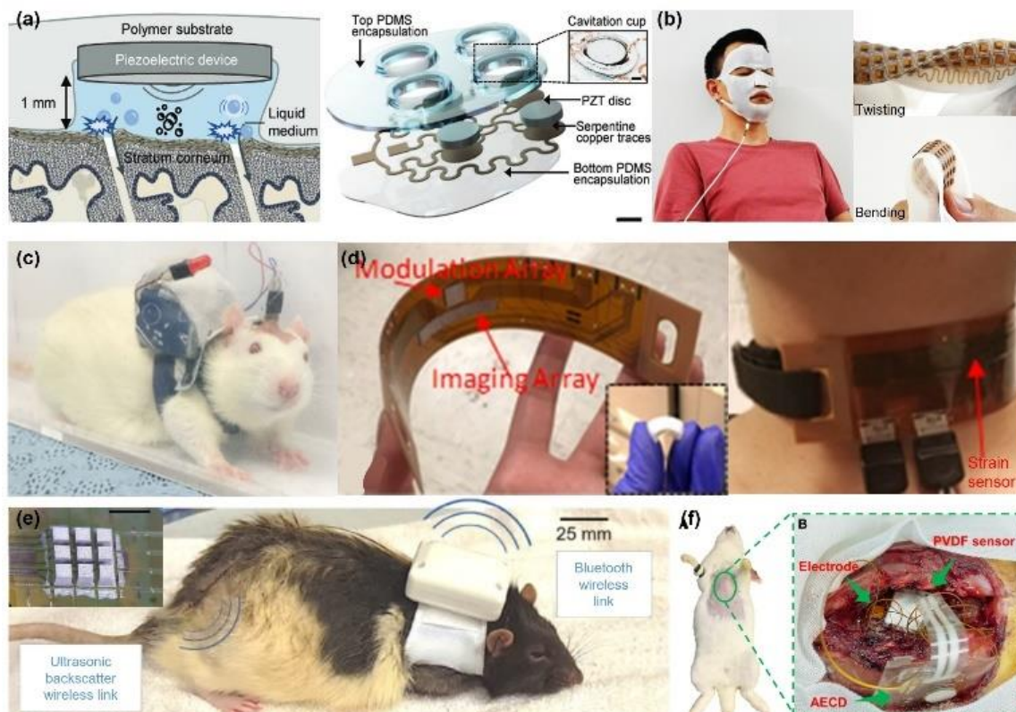
Fig. 3. Wearable ultrasound enabled drug delivery and human-machine interfaces. (a) A conformable ultrasound patch for cavitation-enhanced transdermal drug delivery (left) and the design of a conformal ultrasound patch (right). Adapted from [102]. (b) A stretchable ultrasound facial mask for sonophoresis. Adapted from [103]. (c) A wearable transcranial ultrasound stimulation device on a freely behaving mouse. Adapted from [104]. (d) A flexible ultrasound patch for peripheral nerve stimulation. Adapted from [105]. Implementing ultrasound-based neural interface in a mouse (e) and a rabbit (f). Adapted from [8] and [106].
